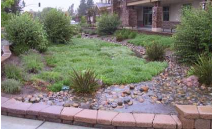
Bioretention facilities can rectangular, linear, or nearly any shape. Photo by Scott Wikstrom
