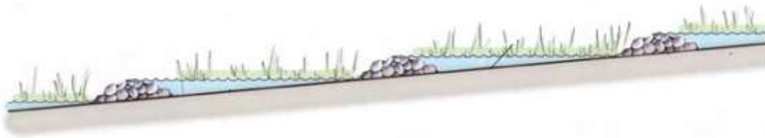
Swale with check dams. Provides limited storage; not suitable for slopes 6% and greater.
